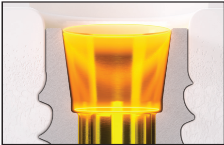
1 7.5° conical connection Tapered Pro Conical's connection features a long conus designed to reduce micromovements and a 7.5° angulation that is proven to provide superior positional stability in comparison to other conical systems. 2
