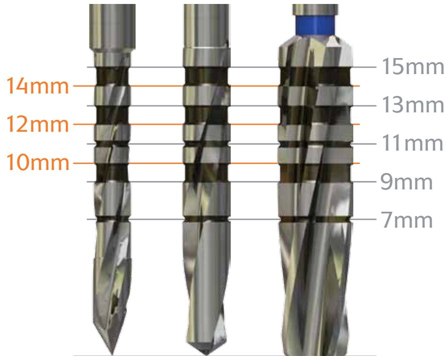
The depth marks are consistent throughout the Starter Drill, Depth Drills and Width Increasing Drills. The thick bands are each one millimeter wide. Thin lines are used to mark 7mm and 11mm.
