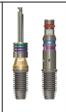
The Surgical Drills included in the External Surgical Kit are externally irrigated and designed to be used at speeds of 850-2,500 rpm<sup>9</sup> with steady sterile irrigation. Reduced drill speed may be desired in softer bone or as drill diameter increases.
