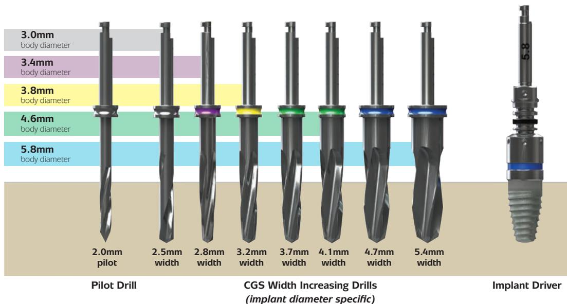
The 2.8mm drill is for the 3.4mm diameter implant, it is not needed for the other sizes. Sold Separately.
