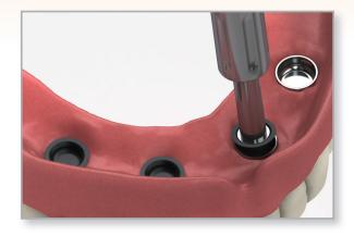
Insert the male removal tool end into the cap assembly and push straight down into bottom of the nylon male. Tilt the tool so the sharp edge grabs the black insert and pull it out of the cap. To discard the insert from the tool, point it down and away from you and tighten the male removal tool clockwise back onto the core tool. The insert will dislodge from the tip of the tool.
