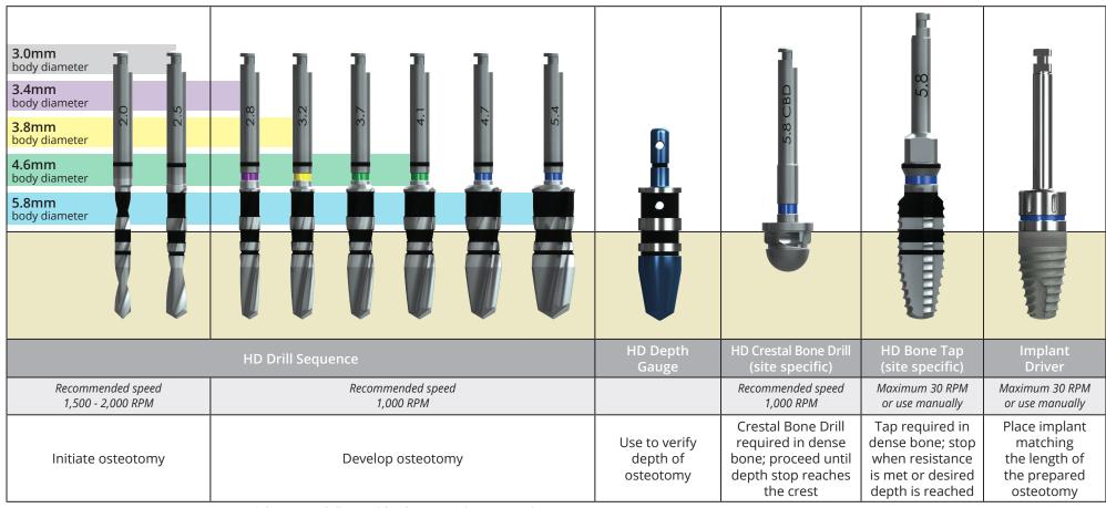
\*The 2.8mm drill is used for the 3.4mm diameter implant, it is not needed for other sizes.
